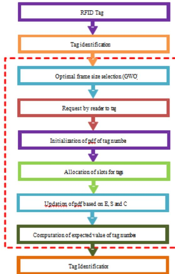
**Fig. 1.** Proposed Tag Anti Collision Method Using BEDFSA
