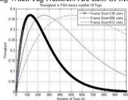
**Fig. 2.** FSA Throughput For Different Frame Size
