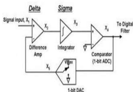
Fig 6.2 Delta-sigma ADC
