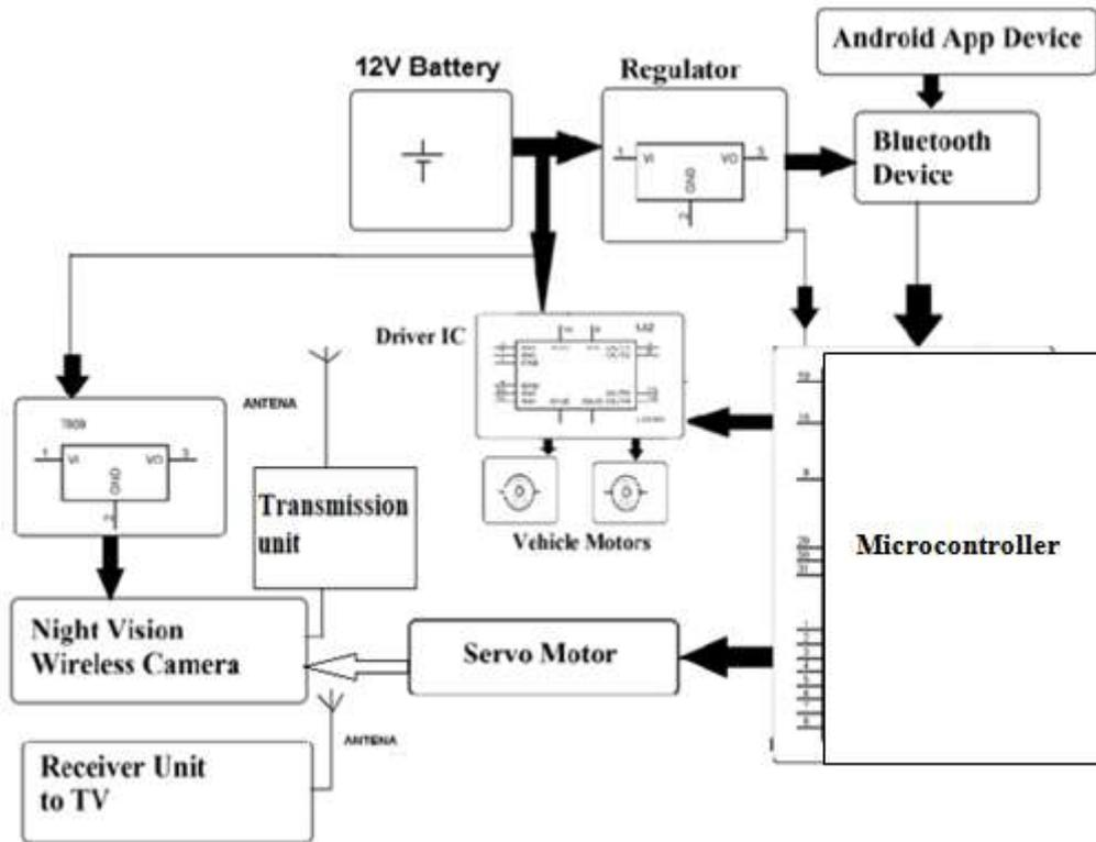
Fig. 1. Block Diagram of Android Controlled Wildlife Observation Robot
