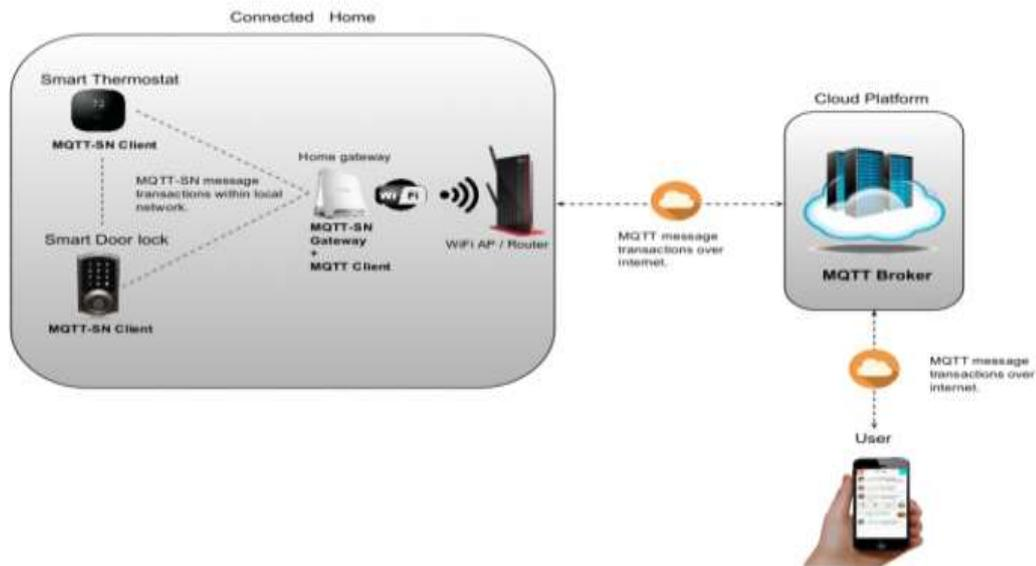
**Figure 2. MQTT-SN and MQTT in Home Automation Example**
