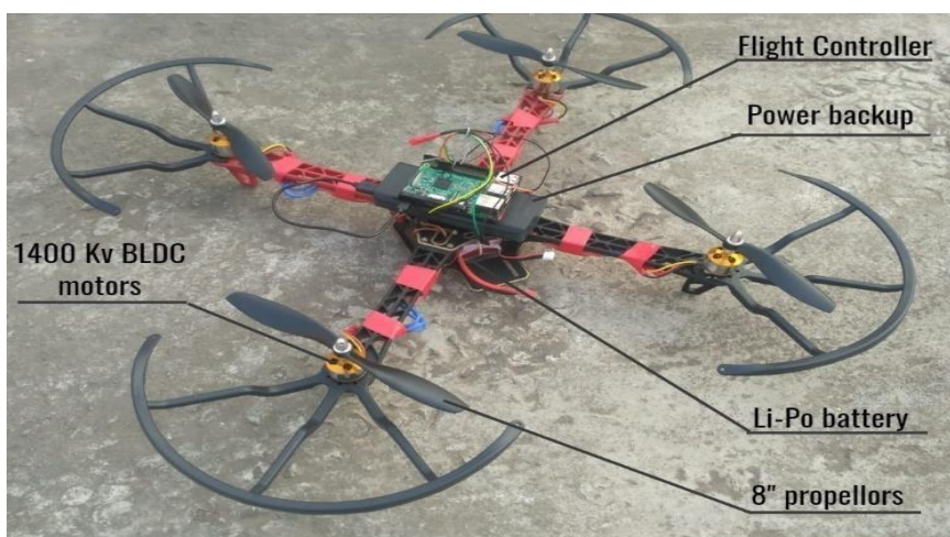
Figure 6. Raspberri Pi 3B based quadcopter model which runs the PID loops and the control signal in the RPI flight controller.
