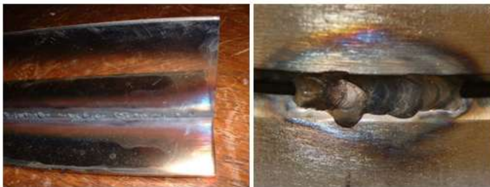
Fig: Porosity & Weld Bed
