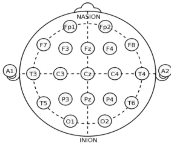
**Figure 1:** International 10-20 EEG system electrodes locations.
