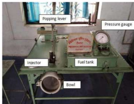
Fig.1(a) MUI testing machine
