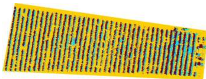
Figure 7. Supervised classified image by using the AdaBoost algorithm by using the G,R,RE,NIR, DSM. Yellow means soil, brown means shadows, cyan represents tree.
