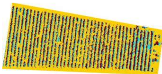
Figure 8. Supervised classified image by using the AdaBoost algorithm by using the G,R,RE,NIR,NDVI and DSM. Yellow means soil, brown means shadows, cyan represents tree.
