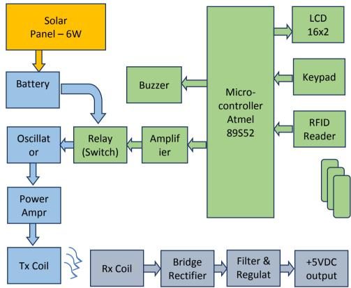
Atmel 89s52 also interfaces with the keypad for typing the charging duration and a secured pin for the payment.LCD is used for display of duration of charging and for the other purposes. Buzzer is provided to give a beep sound after the charging is completed. So the user can disconnect his device.
