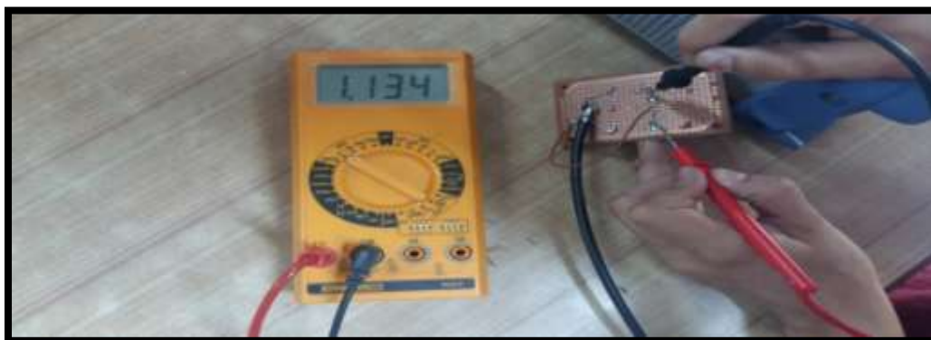
Fig.IV.1 Experimental Setup For Testing Rectifier Circuit To Be Used In RF Harvester
