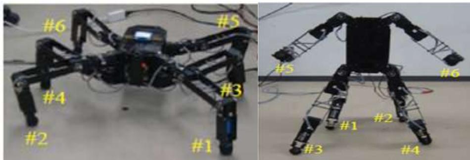
Figure 4: Six-legged mode (left) vertical four leg two arm mode(right)
