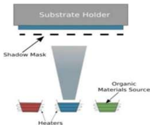
Figure 3. Evaporation and shadow masking
