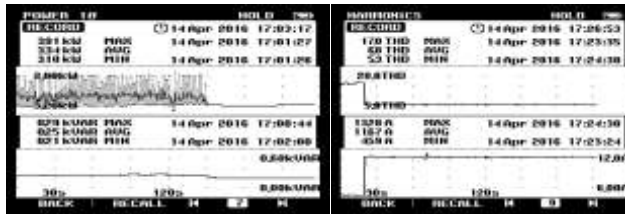
Fig.10. Power consumption & THD monitoring in between 10:00am to 02:00pm
