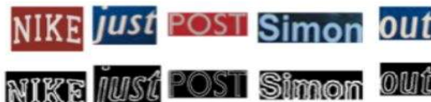
Fig:2.1 Stroke Width Transform
