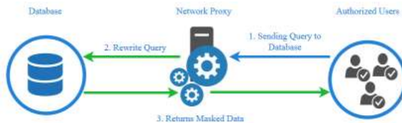
Fig. 3: Conceptual diagram of Request Based Dynamic Data Masking
