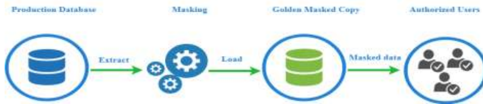
Fig. 2: Conceptual diagram of Static Data Masking
