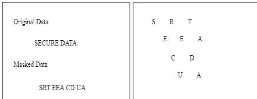
Fig. 6: Example of Rail-Fence Method
