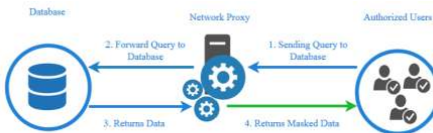
Fig. 4: Conceptual diagram of Response Based Dynamic Data Masking
