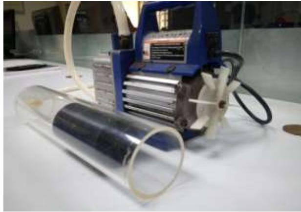
Fig. 1 Tube with Evacuation Setup
