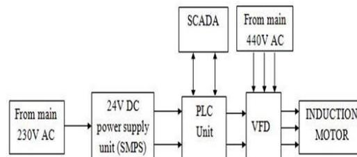
Fig Block Diagram
