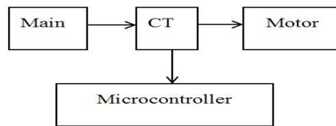
Fig.- Current measurement
