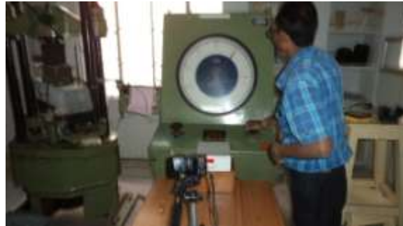
Fig. 2.9 Load frame and test setup for flexural test
