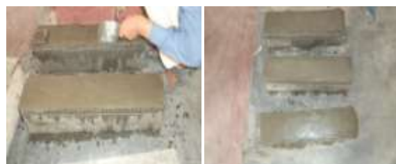
Fig. 2.8 covering of ferrocement jacketing on beam specimen
