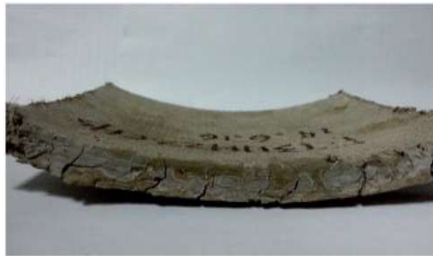
Fig. 6. Over-expansion cracks induced by extra amount of calcium sulfate in CSA cement with mixing.
