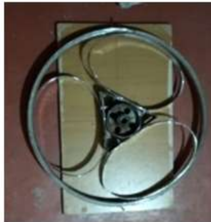
Figure 12 :- Preparation of In-Wheel Loop Suspension System.
