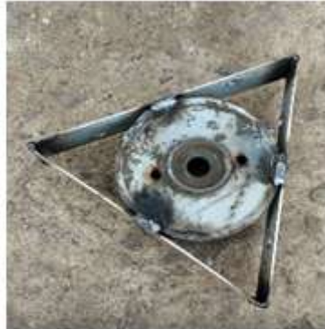
Figure 11 :- Mounting of plate over Drum.
