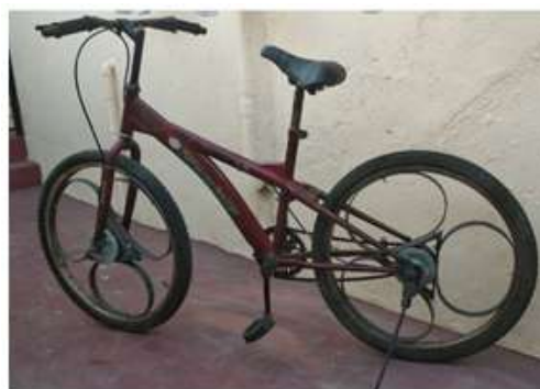
Figure 13 :- Complete In-Wheel Loop Suspension System in Bicycle.
