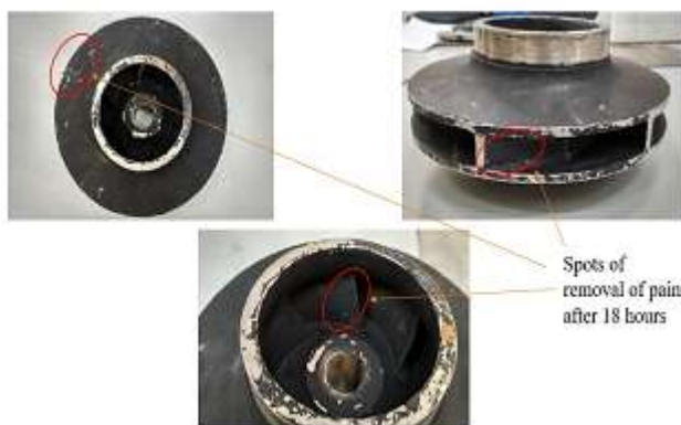
Fig. 5(a) Silt erosion impact areas[16]
