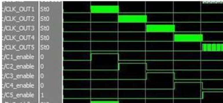
The Partitioning Of The Source Clock With The Reconfigurable Clock Divider Contributes To The Improvement Of Clock Speed In The New Design. Also The Hardware Matching Engine Only Uses A Few Percents Of The Luts Available In The FPGA Board.
