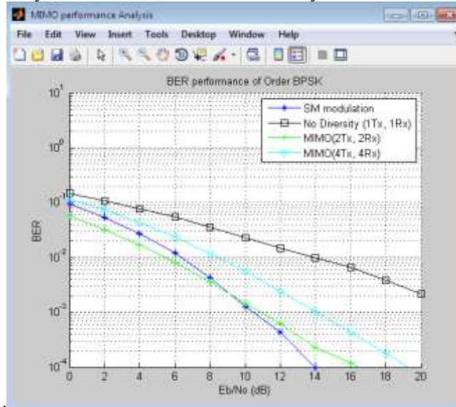
Fig. 2: MIMO Vs. IM Modulation
