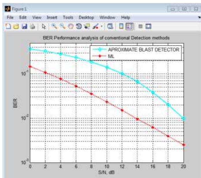
Fig. 4: Performance Of ML Over Conventional Detectors
