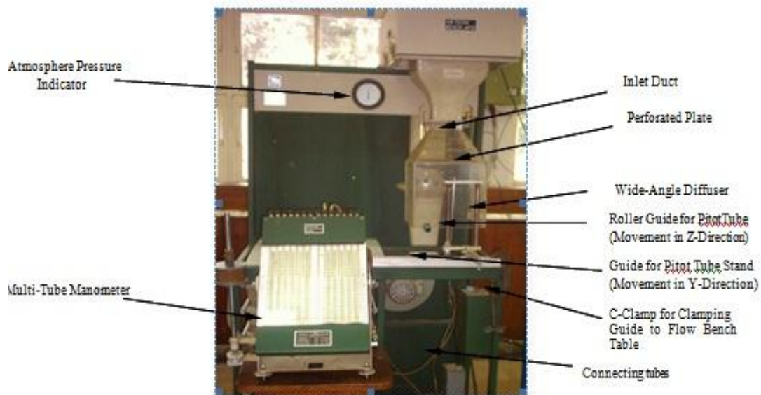
Figure 1. Actual Experimental Setup for Velocity Readings
