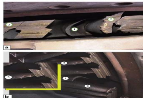
Fig.2.2. Position of the failed blade and the damages were caused due to failure.
