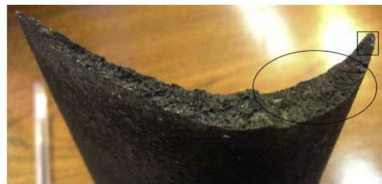
Fig. 2.9 General view of the fracture surface.
