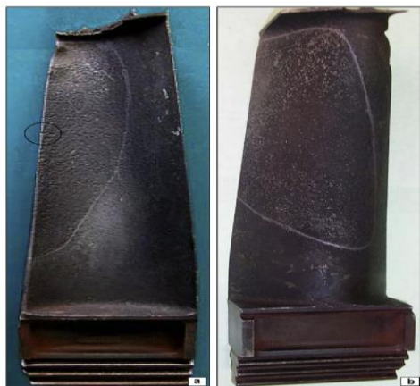
Fig. 2.3 General view of the blade number 3 showing corroded regions. (a) Concave surface. (b) Convex surface.
