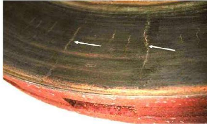
Fig.2. Thermal Cracking In Disc Brakes[2]
