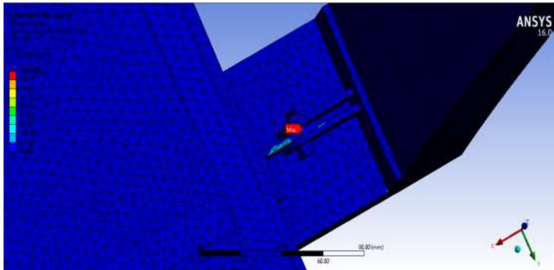
**Fig. 12:-** Location of maximum Stress Concentration (Hinges)
