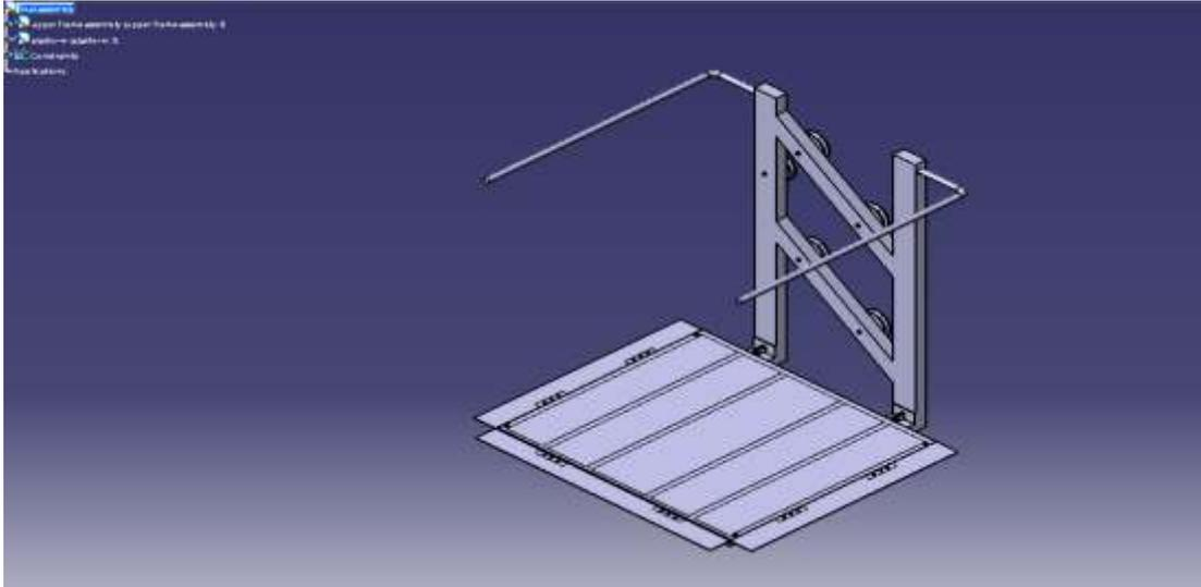
**Fig. 7:-** Isometric view of Platform Stairlift model
