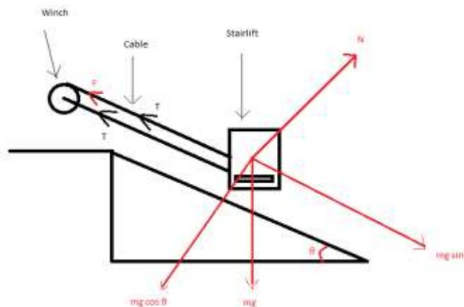
**Fig. 6:- Force Components acting on the stairlift**
