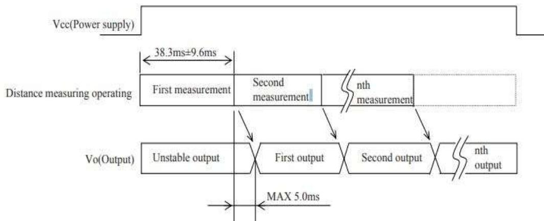
Fig. 5:-Timing Chart of IR Sensor [6]
