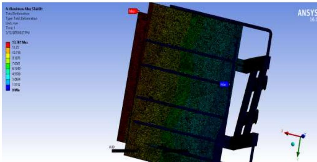
**Fig. 10:-** Total Deformation analysis.
