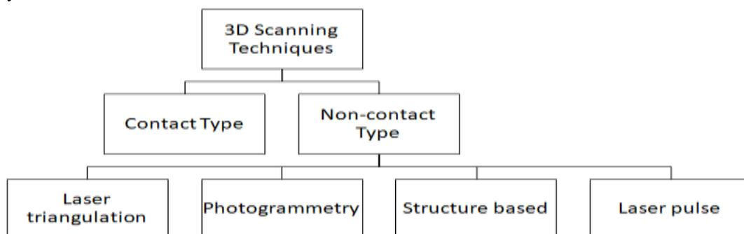
Fig. 1 Classification of 3D Scanning Techniques
