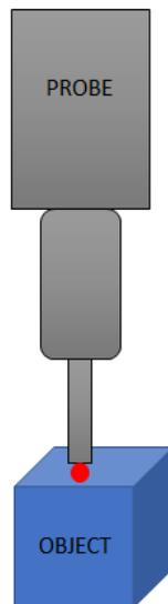
Fig.5 Contact Based 3D Scanning.
