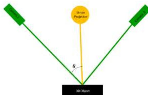
Fig. 3 Structured Light 3D Scanning
