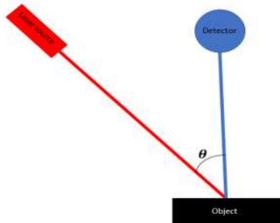
Fig. 2 Laser Triangulation Technique
