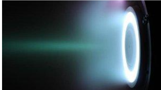
Fig 5. Thruster with Xenon Propellant
