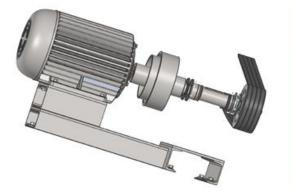
Drive pulley is 3-inch diameterwith 3 no of grooves.
