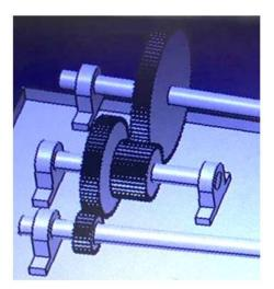
1<sup>st</sup> stage reduction: No. of teeth of pinion is 27 No. of teeth of wheel is 76 Centre distance between two gear is 80 mm PCD of pinion is 40 PCD of wheel is 120 Transmission ratio is 2.814
