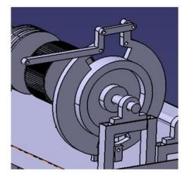
Total Torque applied on shaft drum (200 mm dia) = Torque on left arm + Torque on Right arm Total design torque = 373 Nm
