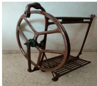
Fig. No. 5: Sewing Machine Pedal Mechanism with Bevel Gear
