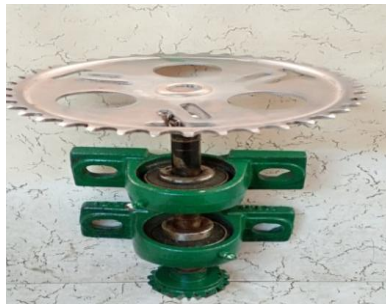
Fig. No. 6: Sprocket with Bevel Gear and Bearing
