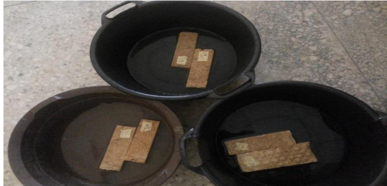
Fig 3.6: Sample soaked inside distilled water
