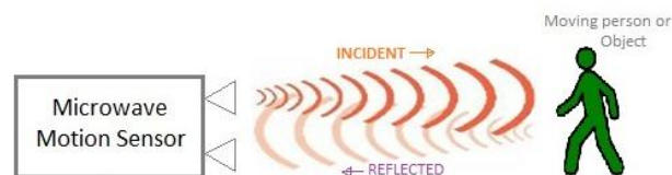
Figure 6.1 Working of Motion Sensor
