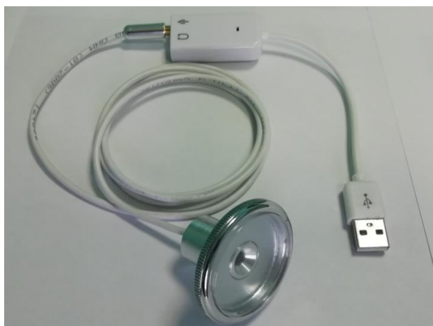
Fig. 1 Registration system based on the microphone Panasonic WM61a and sound card DEXP 3D CM108 USB 2.0.
