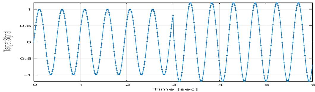
**Figure 11** Recovery signal to boost the voltage during dip
