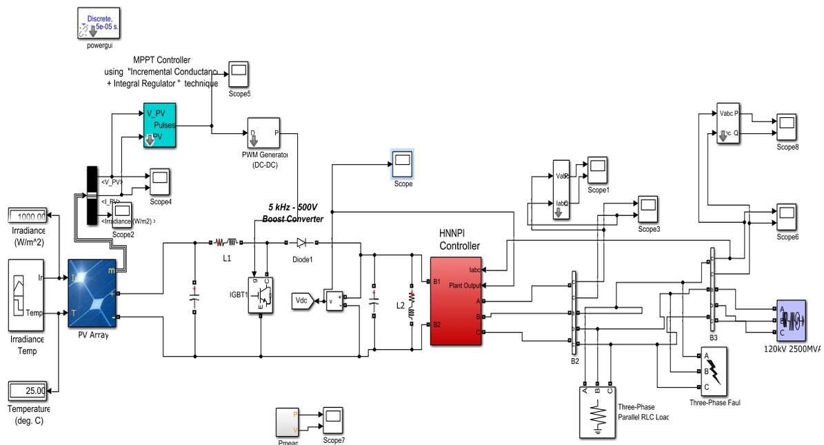
**Figure 4** Matlab model of proposed MNNPI based GCPVS
