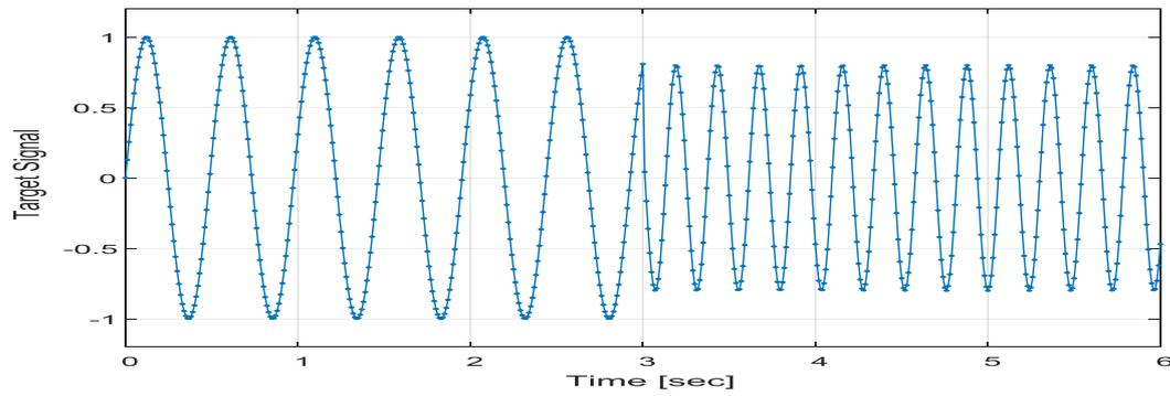
**Figure 10** Output signal of NN during voltage dip grid side
