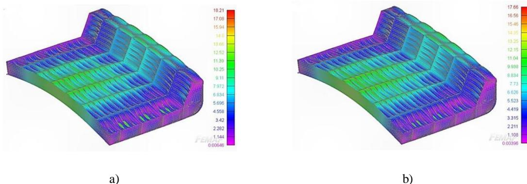
**Figure 14** The case of settling on the wave ridge, the displacements that appear in the complete 3D-FEM model
