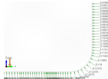
**Figure 6** Distribution of hydrostatic water pressure on the outer shell
