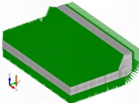
**Figure 7** Distribution of hydrostatic pressure of the goods and water on the inner and outer shell
