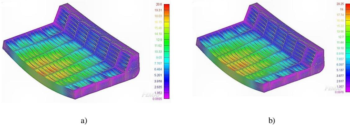
**Figure 12** The case of placing on a wave gap, the displacements that appear in the complete 3D-FEM model
