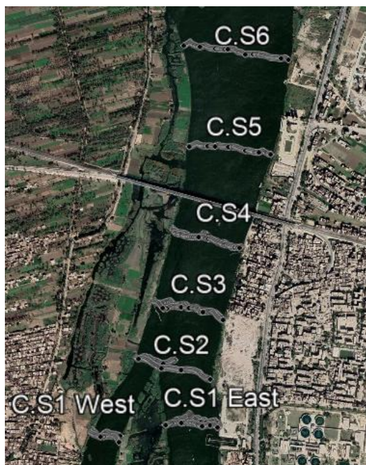
Figure 2: ADCP data points along the study reach during the field measurements at year 2019
