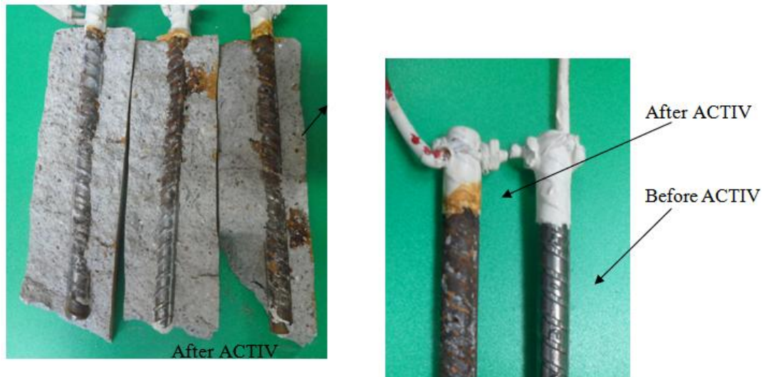
Figure 6. Reinforcement Steel after ACTIV.
