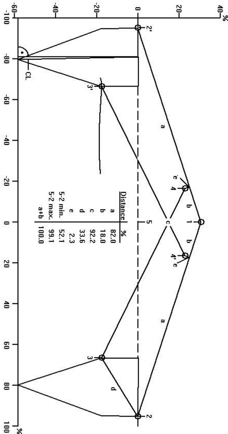
Fig. 3. Folding mechanism for a catamaran keeping the hulls virtually upright (see text)
