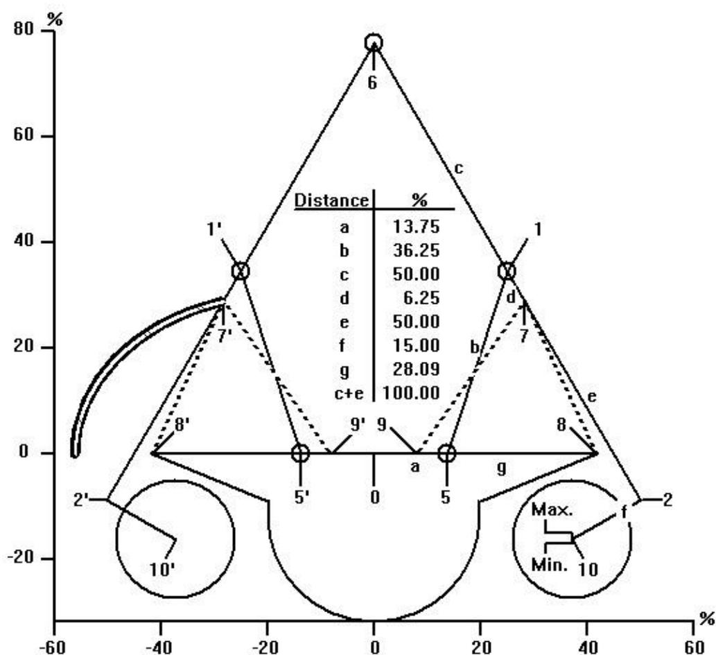
**Fig. 2.** Folding mechanism with 2 hinges on a trimaran main hull (see text)
