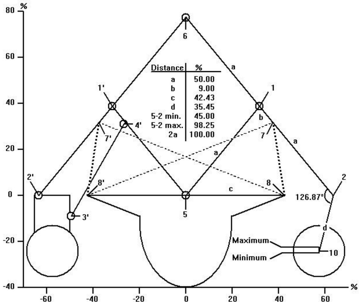
Fig. 1. Folding mechanism with 1 hinge on a trimaran main hull, right float rotating, left float fixed.(see text)
