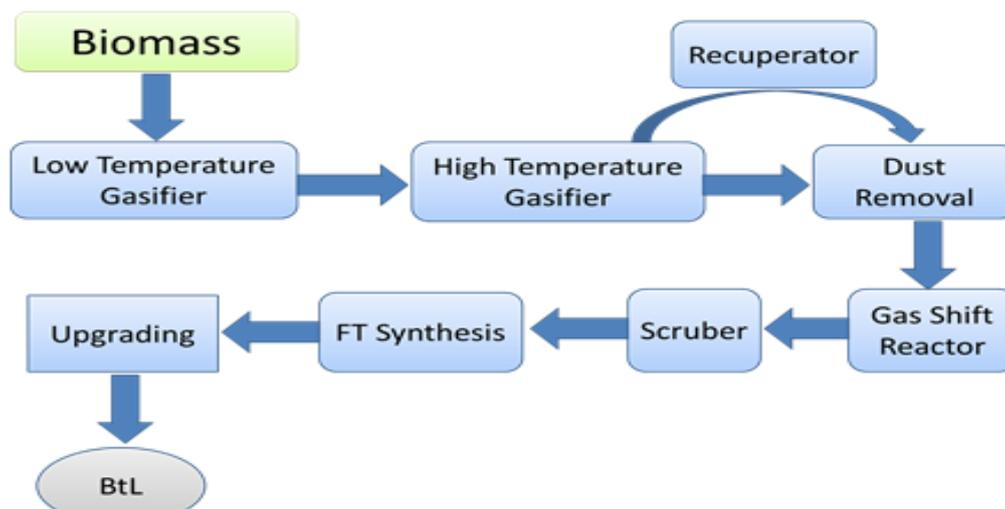
The main catalytic process to convert the syngas into a liquid fuel is known as Fischer-Tropsch (FT). This process occurs at high temperatures; it consists of a reaction between hydrogen and carbon monoxide that is explained by the following equation:
