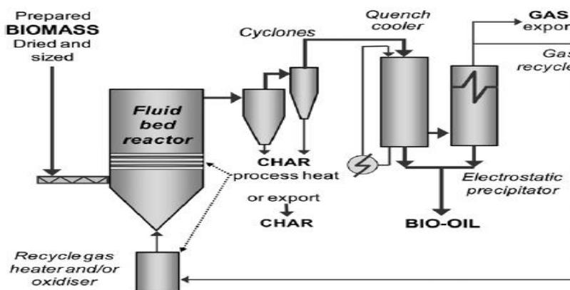
Scheme of the Fast Pyrolysis Process
