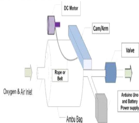
Figure 8: Working Process of Setup
