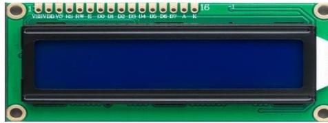
Figure 3: 16x2 LCD Module
