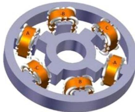
Figure 4: Stepper Motor
