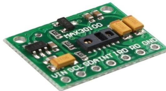
Figure 7: Blood Oxygen Sensor
