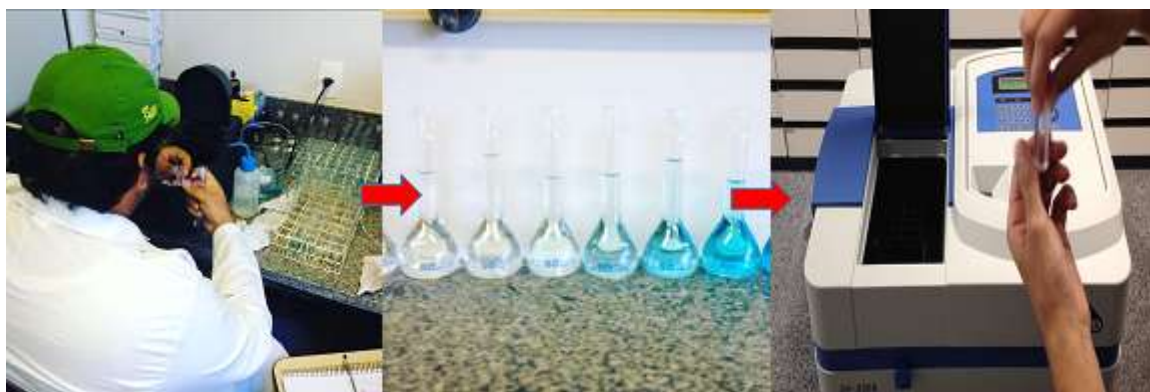
Figure 2. Tracer dye deposition analysis from sample preparation to spectrophotometer analysis
