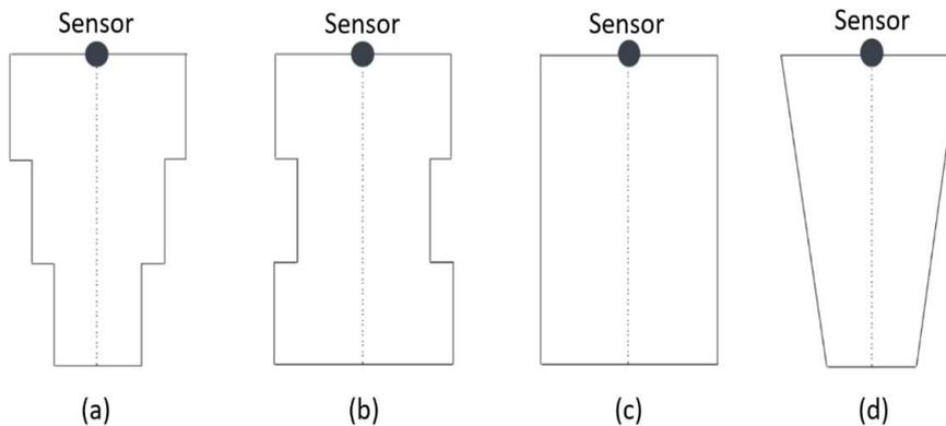
Figure 5: Sensor mounting position, and shape of the trash bin. Bins (a) and (b) are not recommended, Bins (c) and (d) are recommended.
