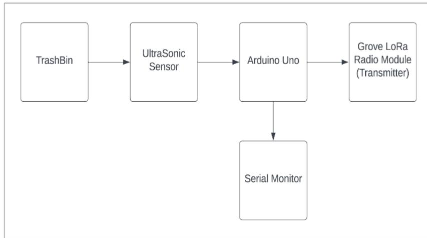
**Figure 2:** Block diagram of the transmitter node.
