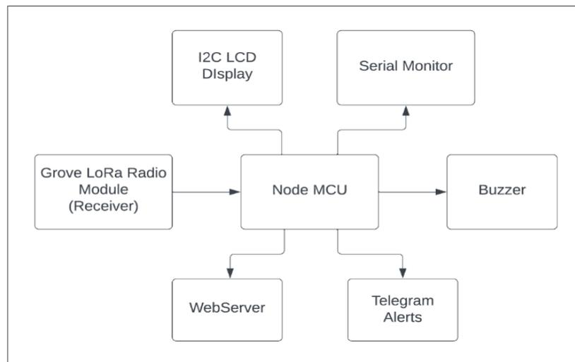
**Figure 3:** Block diagram of the receiver.
