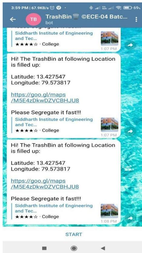
Figure 12: Alerts using Telegram along with location, when trash level in bin is filled above 90%.
