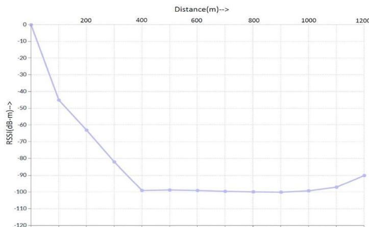
**Figure 7:** RSSI vs Distance plot
