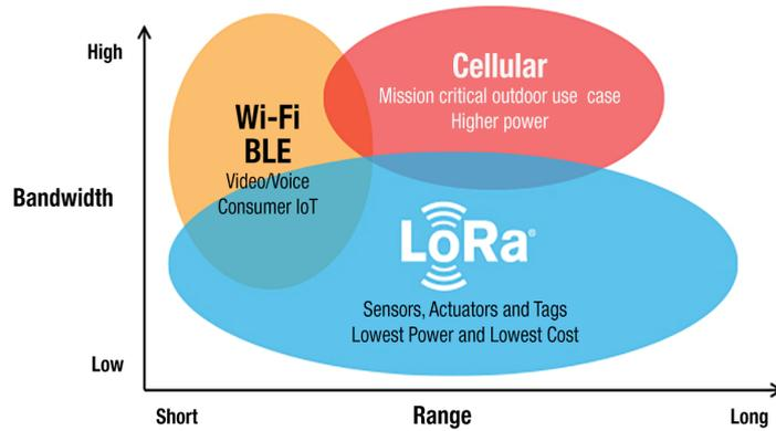
Figure 4: Bandwidth vs Range of Some Communication systems.
