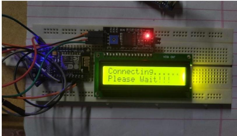
**Figure 9:** Device status while connecting to Wi-Fi.
