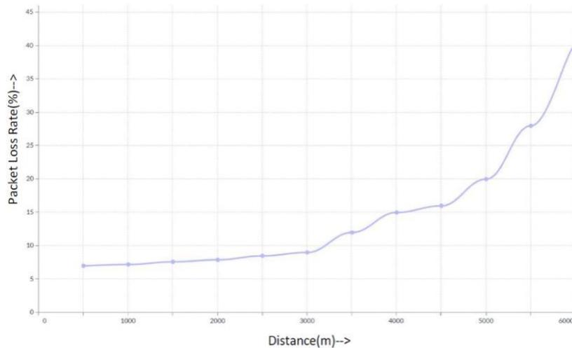
**Figure 6:** Packet Loss Rate vs Distance plot
