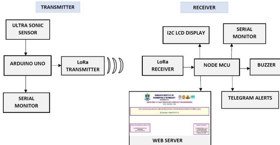
Figure 1: Block diagram of the total system.
