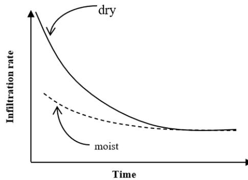
**Figure1.**Ideal Infiltration Curve
