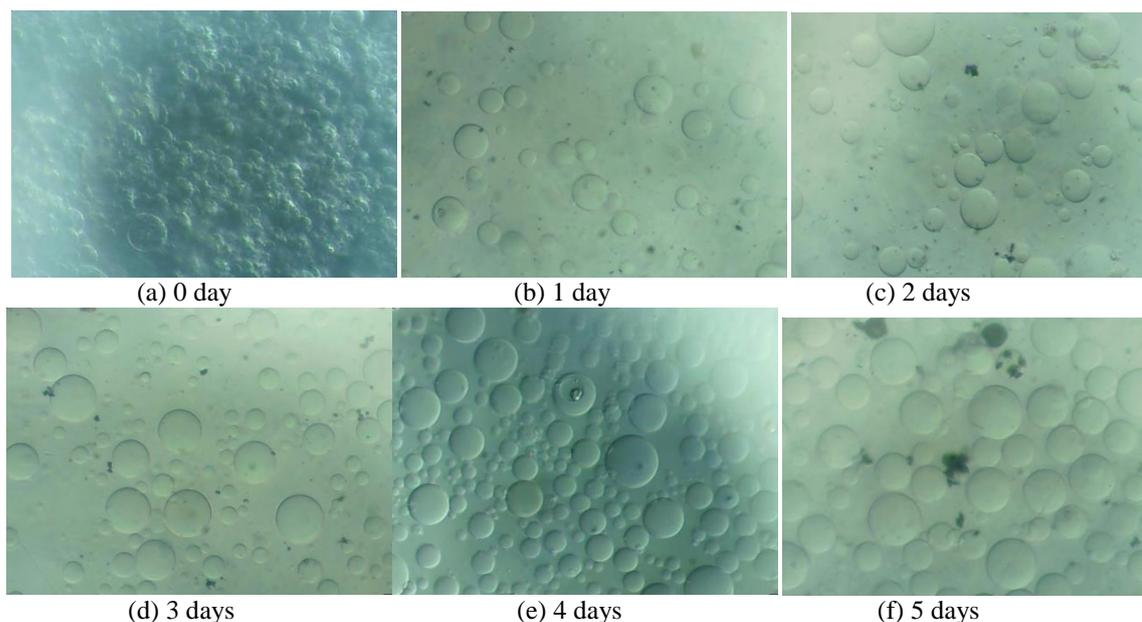
Fig.4 Hydration swelling of MDS /dy-2 solution
