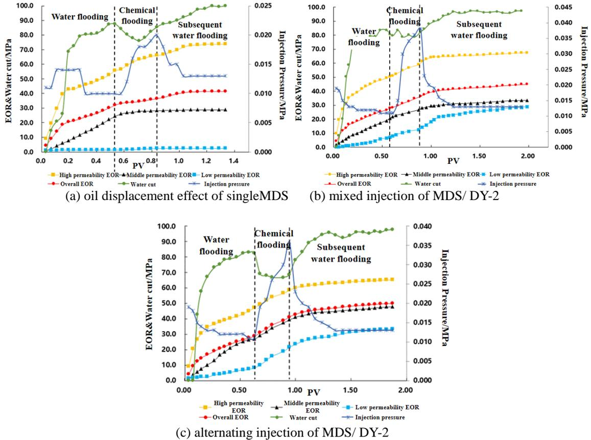
Fig.8 Dynamic characteristic curve of injection mode optimization
