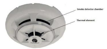
**Optical smoke detectors-** This detector consists of a light source and a photocell positioned at an angle to each other. In normal conditions the transmitted light passes into a "light maze" which prevents the reflection of light onto the receiver. In the event of fire, the passing fumes through the detector scatters the light onto the photocell and at a specific threshold value of light intensity the detector activates.
