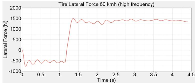
**Figure 5.** Lateral Force at 60 km/h.
