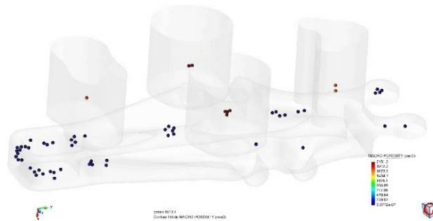
**Fig 17.** Cast Simulation filling process – porosity volume
