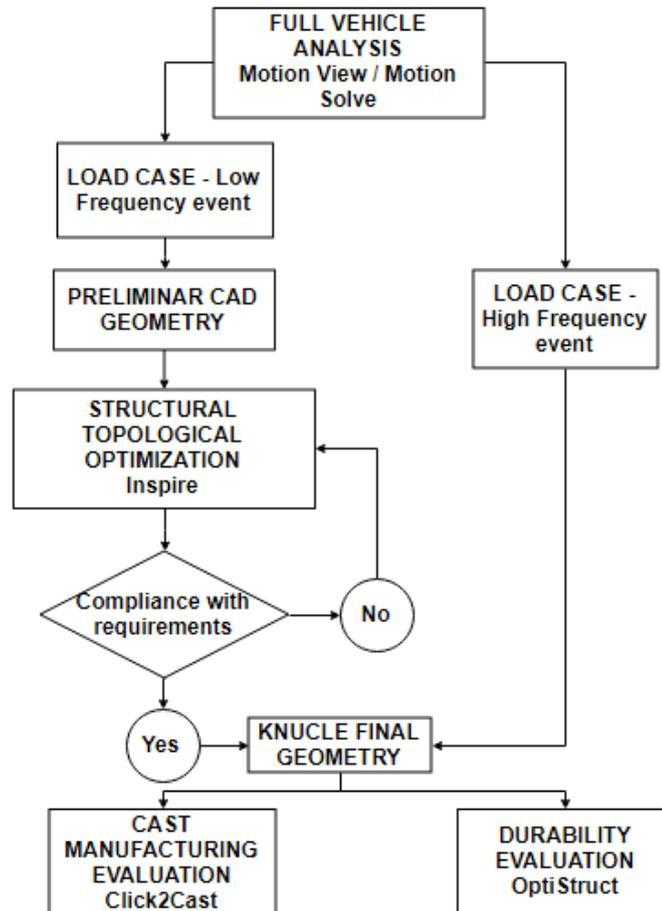
**Figure 2.** Simulation Based Design Workflow.
