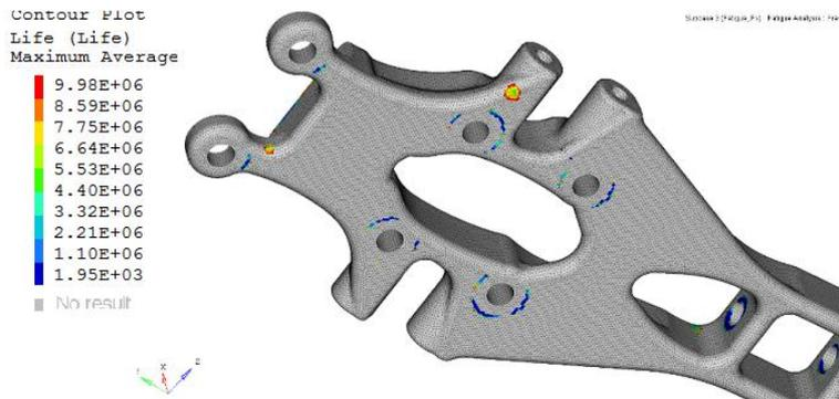
Figure 15. Fatigue Life Results (the color blue is the warning zone with less life cycle)
