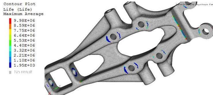
Figure 14. Fatigue Life Results (the color blue is the warning zone with less life cycle)
