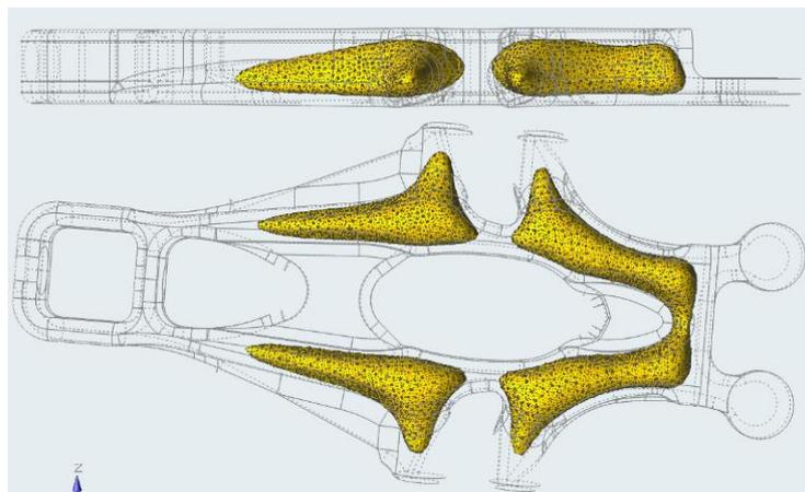
Fig 16. Cast simulation solidification process, final zone.
