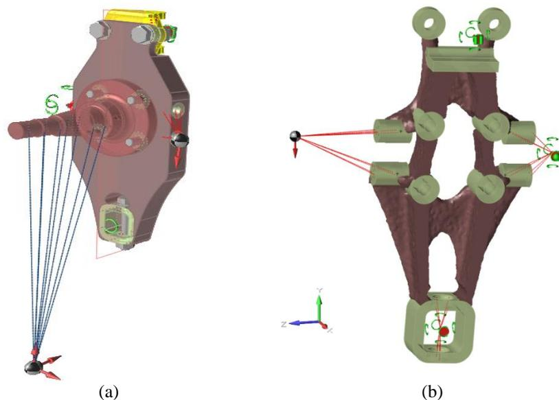
**Figure 8.** (a) Inspire FEM Model, (b) Optimized Shape in Inspire Simulation.
