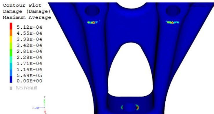
Figure 13. Fatigue Damage Results
