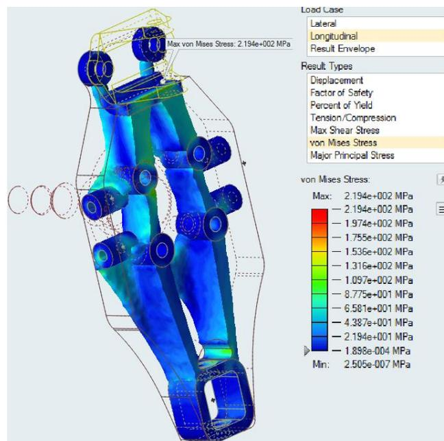
**Figure 10.** Braking results.
