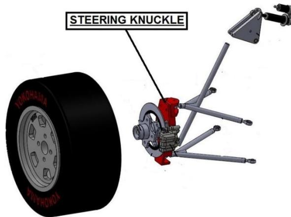
**Figure 6.** Baseline assembly for steering knuckle mount.
