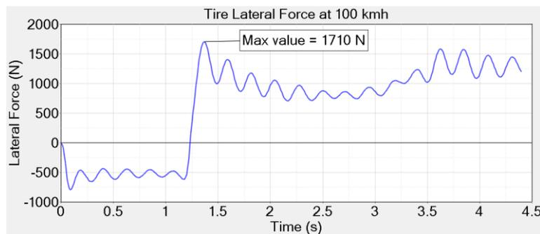
**Figure 4.** Lateral Force at 100km/h.
