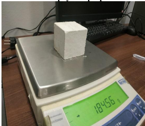
Image (29) shows Weighing samples to estimate their physical properties
