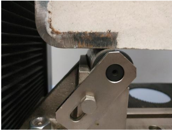
Image (39 ) shows supporting pins before testing
