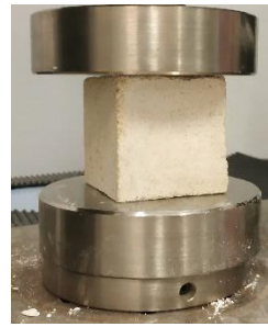
Image (34 ) shows the compression test of sample No. 2 (5 cm3) after salt aging and in a wet condition
