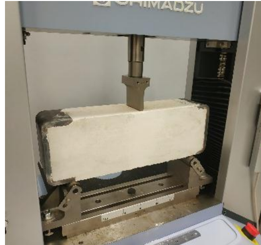
Image ( 40 ) shows loading pin before testing
