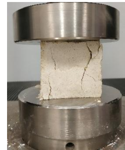
Image (35) shows the collapse of sample No. 2 after salt aging and in a wet condition
