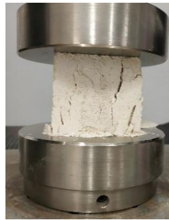
Image (33) showing the collapse of the cube Sample1
