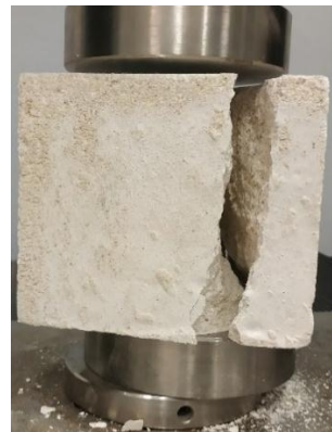
Image ( 37) showing the collapse of the cube Sample3
