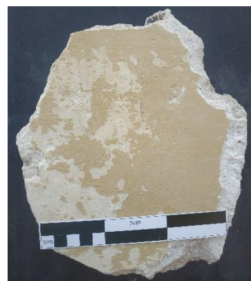
Image (12) of the layers of render and colors on the concrete sample
